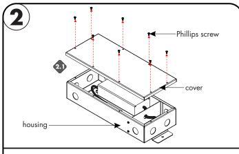
2.1 Remove the eight Phillips screws from the top of the driver housing and pull the cover off to expose the driver wires.
