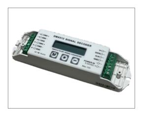
The SR-DMX-SPI is a smart LED pixel decoder that controls RGB/RGBW pixel LED strips with SPI signal.
