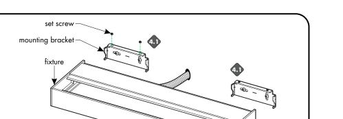
4.1 Bring in the power wires into the fixture . Align the fixture to the mounting brackets and secure in place using the 2 set screws for each mounting bracket. Use the provided conduit connector if
