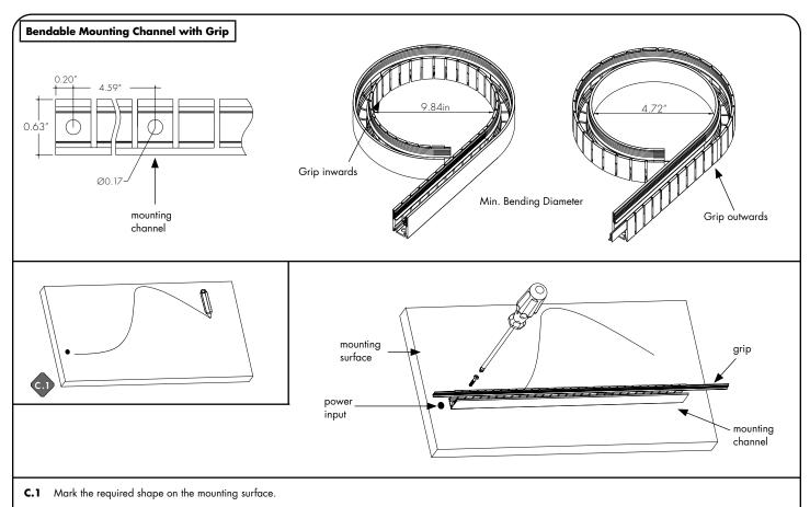
**C.2** Fix the screw starting from the power input end. Keep some distance between the channel and power input.
