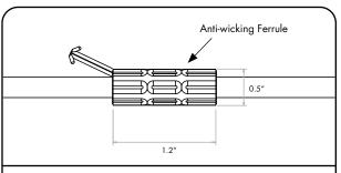
The removal of anti-wicking ferrule will increase the risk of water ingression and void the warranty out of it. For underwater application, do not immerse antiwicking ferrule in the water.
