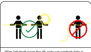
When light length longer than 6ft, make sure somebody helps to lift the light, in case the heavy weight of light itself generates too small bending angle or twisting, which may damage Kurba.
