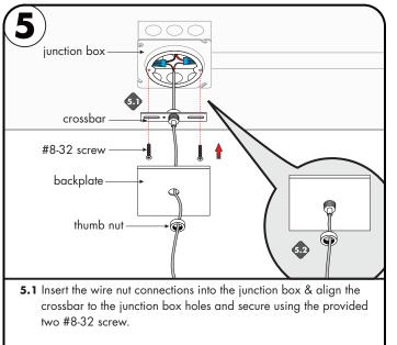
**5.2** Slide the backplate up to the crossbar and secure by hand tightening the thumb nut into the crossbar.
