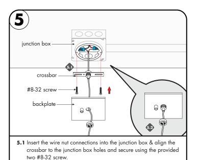
**5.2** Slide the backplate up to the crossbar and secure by hand tightening the thumb nut into the crossbar.
