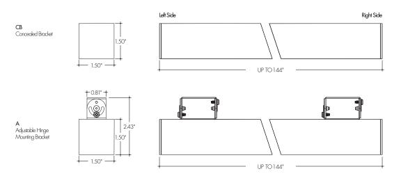
Adjustable Hinge Mounting Bracket is not available on system runs with corners
