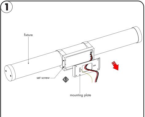
**1.1** From the back of the fixture, loosen the 4 set screws on the fixture body. Then carefully remove the mounting plate.
