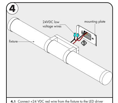
+24 VDC red wire with a wire nut. Connect -24VDC black wire from the fixture to LED driver -24VDC black wire with a wire
